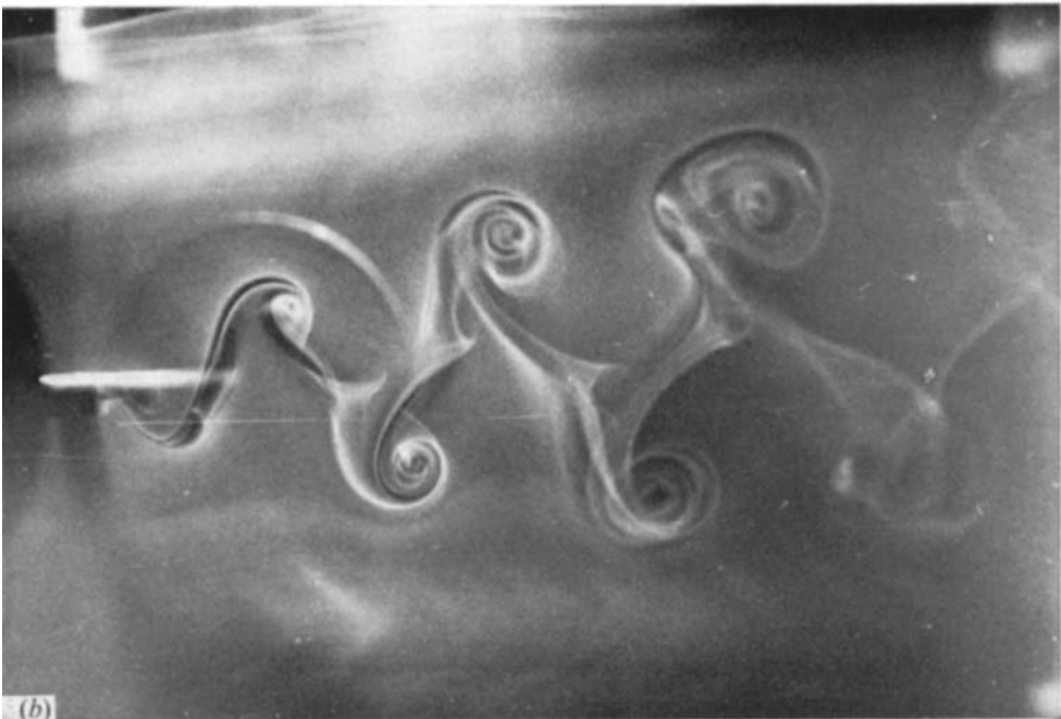
FIGURE 5. Vortex shedding from a cylinder vibrating in line with an incident flow at a Reynolds number of 190. Two vortices were shed during each cycle of the cylinder's vibration. (a) f/f_s = 1.74 , (b) f/f_s = 1.92 .
