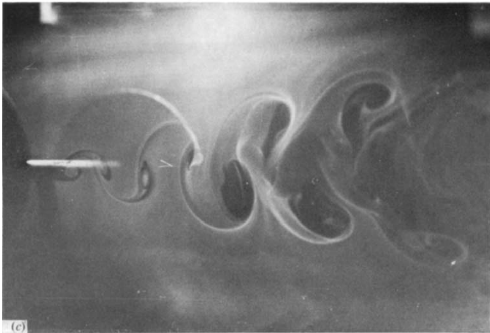
FIGURE 4. The effects of frequency on the vortex wake of a cylinder vibrating in line with an incident flow at a Reynolds number of 190. A single vortex was shed during each cycle of the cylinder's vibration. (a) f/f_s = 1.76 , (b) f/f_s = 2.06 , (c) f/f_s = 2.20 .
