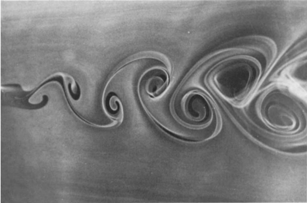
FIGURE 3. Flow visualization of the wake of a stationary cylinder at a Reynolds number of 190. Strouhal frequency f_s = 36.6 Hz, cylinder diameter d = 4 mm, Strouhal number = 0.19.
